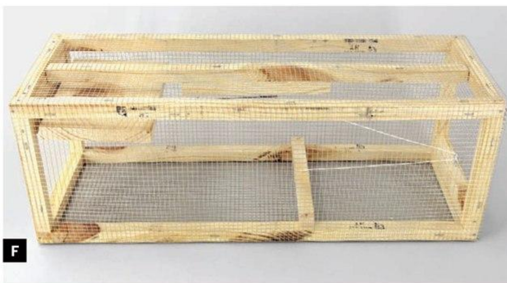
music wire. Fig. D: The latch is just a length of music wire with a loop in one end. Fig. E: Staple the hardware cloth to the cage frame. Fig. F: Run the string from the latch through the medium screw eye, then tie it off.
