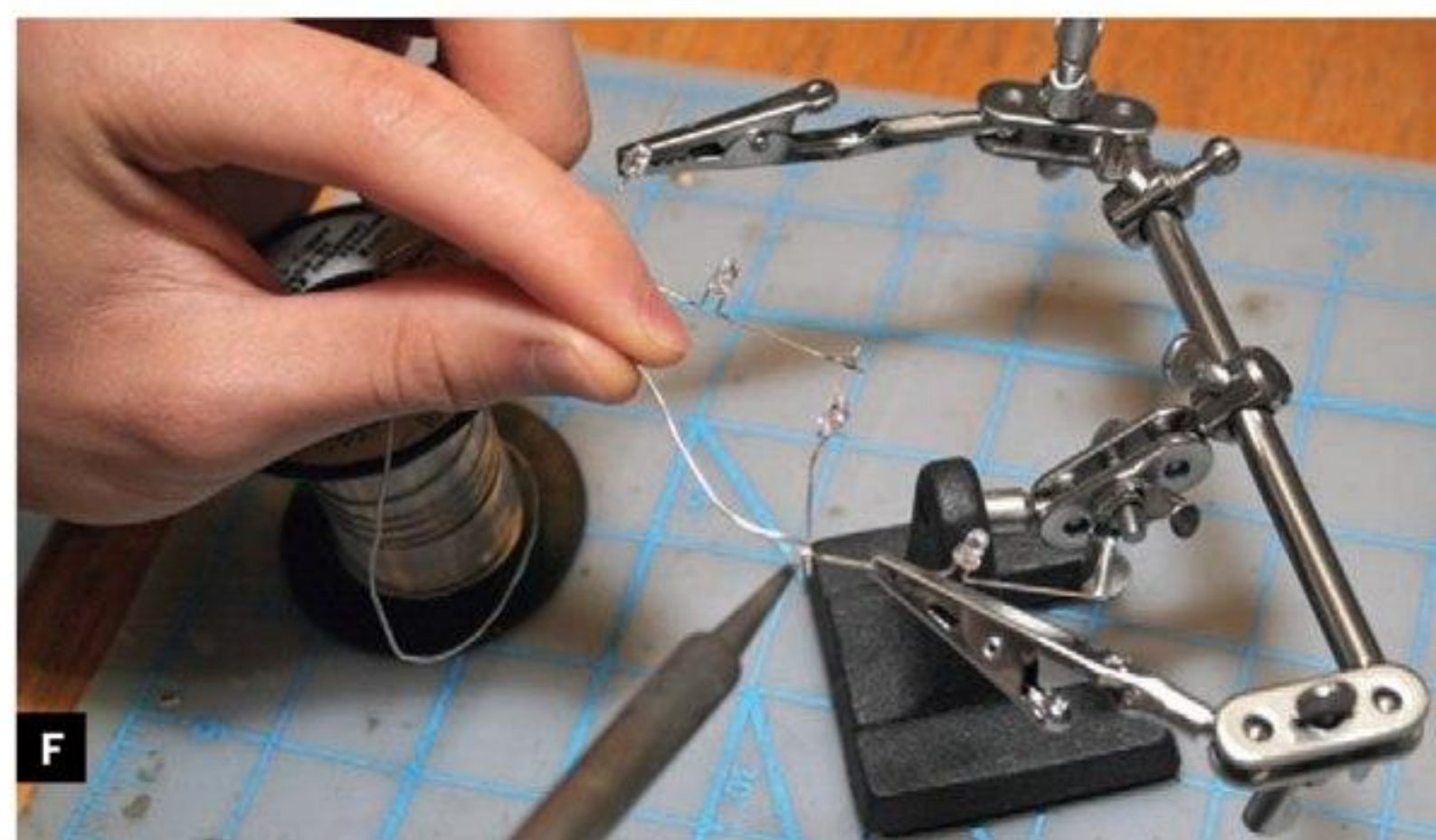
Fig. E: Schematic diagram for the entire circuit, including LEDs and fan. Fig. F: Solder the LEDs together in series with the resistor, or just twist the connections together if you don't feel like soldering.
