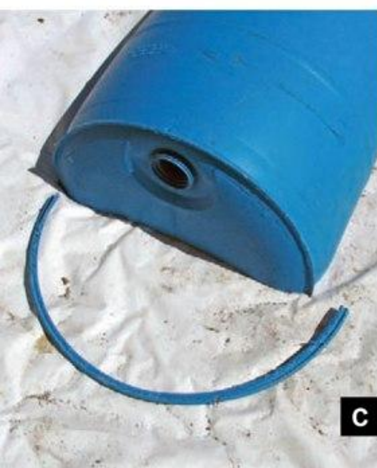
Fig. A: Saw the 55gal barrel in half lengthwise, making sure that the half you use for your hive has a bung-hole. Bees will use it as an entrance to the hive. Figs. B–C: Trim away the protruding rim of what used
