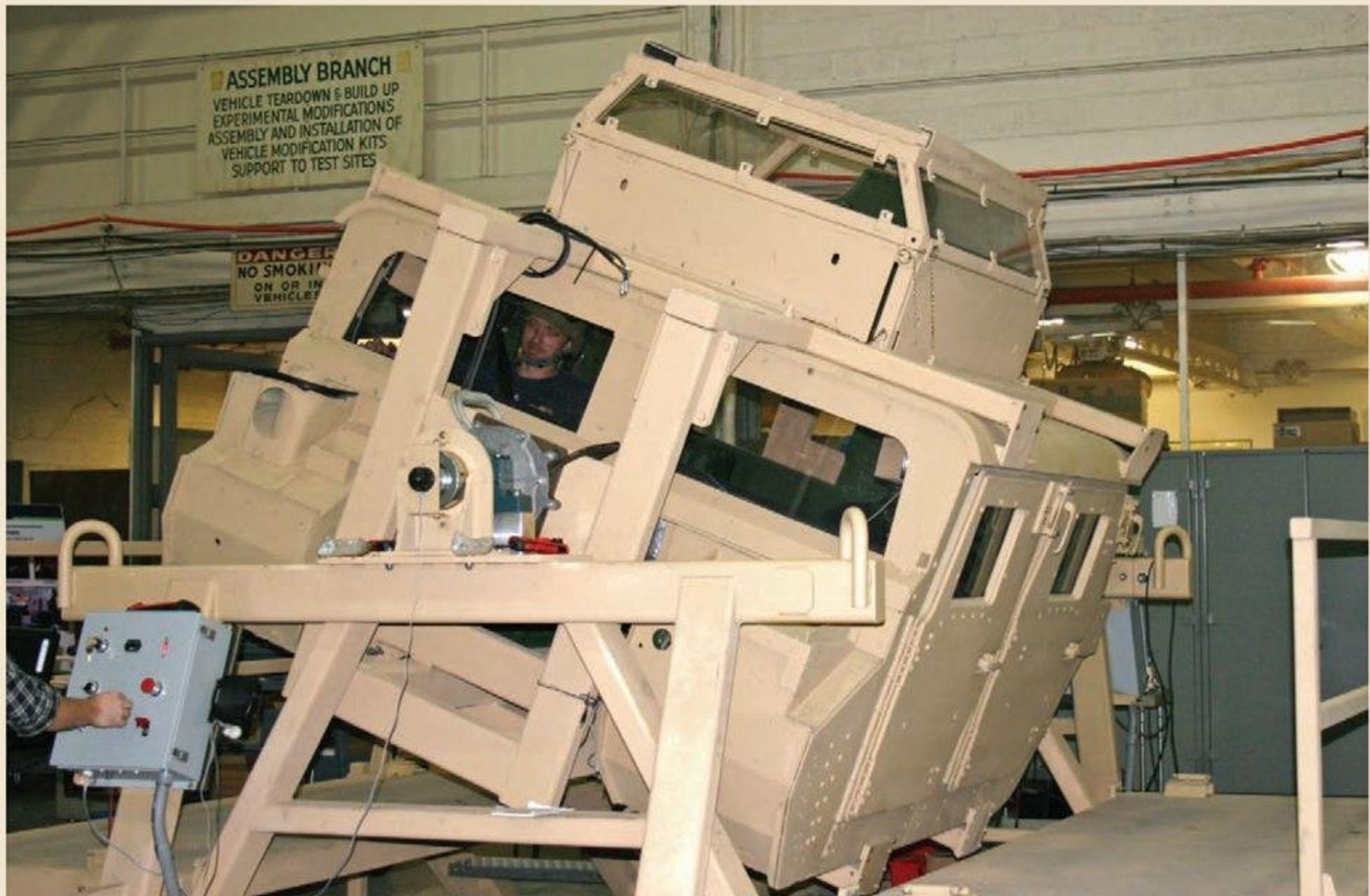
SHAKE IT, DON'T BREAK IT: (Above) The “egress assist trainer” rollover cage was originally designed for training personnel to escape from flipped Humvees. (Below) Overhead Wire Mitigation (OWM) kits let armored vehicles lift wires that are strung across roads out of the way, rather than breaking them.
