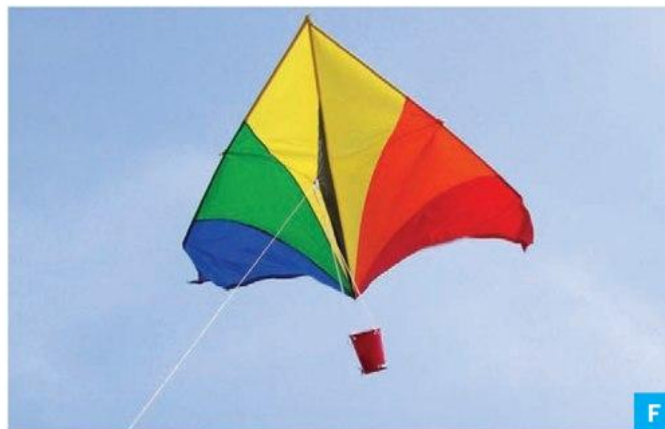
Fig. E: This scatter graph shows an association of mold spores and carbon particles (smoke) collected on microscope slides during 13 days when smoke from Yucatan drifted over South Texas. Fig. F: A DIY passive air sampler flies from a delta kite at Padre Island, Texas, to capture spores in smoke from agricultural fires in Yucatan. Fig. G: At the bottom of the air sampler, binder clips hold the microscope slide in place. Fig. H: Sarah Mims inspects microscope slides for dust, smoke, and spores.
