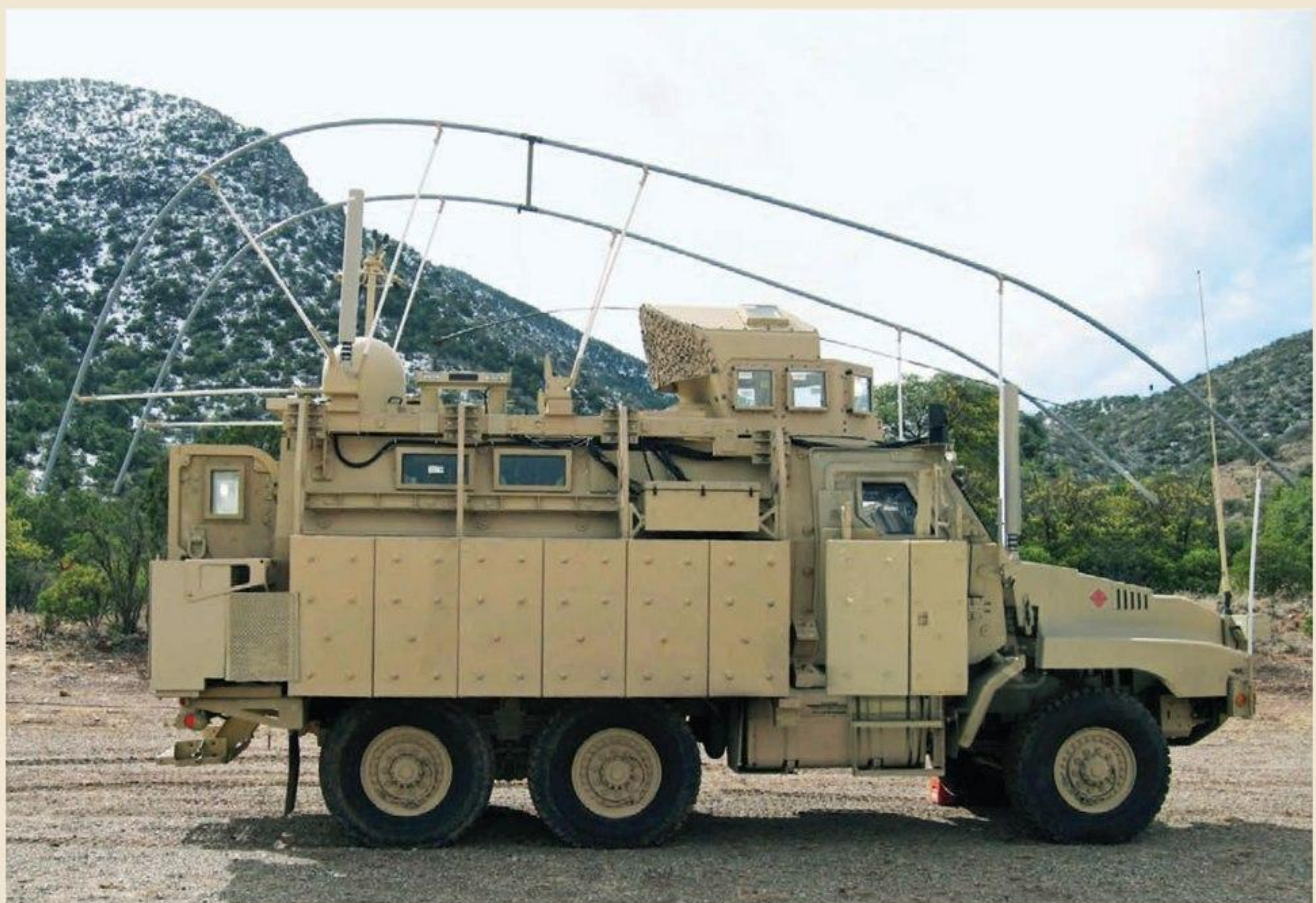
SHAKE IT, DON'T BREAK IT: (Above) The “egress assist trainer” rollover cage was originally designed for training personnel to escape from flipped Humvees. (Below) Overhead Wire Mitigation (OWM) kits let armored vehicles lift wires that are strung across roads out of the way, rather than breaking them.
