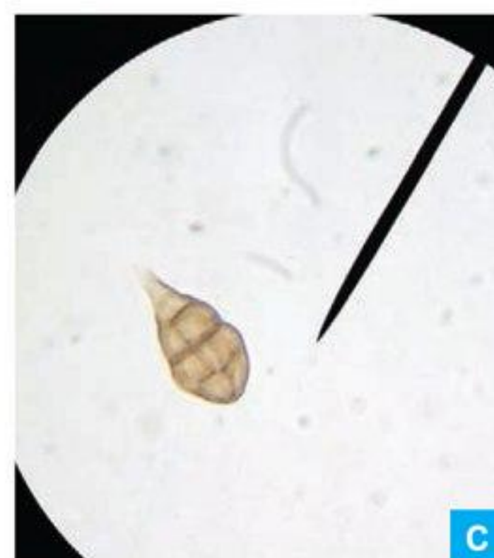
Fig. A: Pollen blowing from a giant ragweed plant, one of the worst causes of hay fever. Fig. B: Pollen accumulates on windshields. Fig. C: Alternaria spore, about 25µm, collected using the sampler. Ragweed pollen is about 20µm in diameter, and human hair 60µm–100µm. Fig. D: Air sampler made from a vacuum cleaner inlet fixture and a microscope slide.
